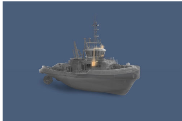
Figure 2: Preferred installation location for sensor unit on tug boats is either mast or on compass deck above bridge. Copyright: Groke Technologies
