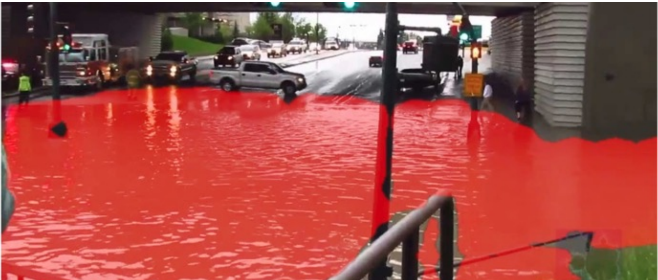
Figure 1. Sample flooding event detection based on the image segmentation model of FloodCAM.
